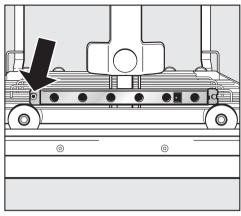
■ Place the track in the holder in the mobile unit and screw firmly in place.
